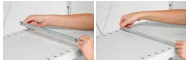
Assembling the guide rails for multibox
