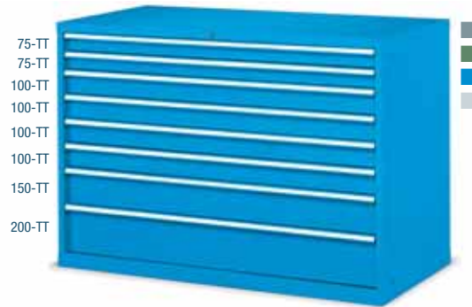
ORD. NO. DRAWERS F AG 7040 02 04 8 Cabinet with 8 full telescopic extension drawers Dimensions mm 1431x726x1000 h Central lock
