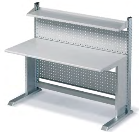
ITEM NO. F LE D125 01 55 ① WORKSTATION DIMENSIONS: 1552x820x1285 mm h COMPLETE WITH: 1 shelf 320 mm - 2 perforated panels - 1 worktop WORKTOP DIMENSIONS: 1470x700x30 mm h WORKTOP LOAD CAPACITY: 200 kg COLOUR GALVANIZED + GREY RAL 7000 + GREY RAL 7035 WORKTOP ADJUSTABLE IN HEIGHT FROM 720 mm to 1138 mm
