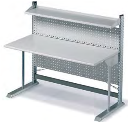
ITEM NO. F LD 0125 01 56 (1) WORKSTATION DIMENSIONS: 1552x820x1285 mm h COMPLETE WITH: 1 shelf 320 mm - 2 perforated panels - 1 worktop WORKTOP DIMENSIONS: 1470x700x30 mm h WORKTOP LOAD CAPACITY: 50 kg COLOUR GALVANIZED + GREY RAL 7000 + GREY RAL 7035 WORKTOP ADJUSTABLE IN HEIGHT FROM 797 mm to 911 mm
