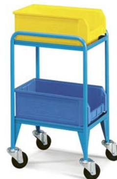
ORD. NO. Dim. mm F CR 0031 03 04 765x560x1030 h Trolley with 2 standard rubber swivel wheels with brakes and 2 standard rubber fixed wheels Ø 125 mm, 1 storage container ORD. NO. F PL 8951 00 03, 1 storage container ORD. NO. F PL 8951 00 05. LOAD CAPACITY: 300 KG
