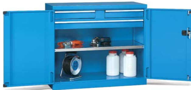
ORD. NO. Dim. mm F AA 1500 55 04 1194x555x1000 h Cabinet with 1 shelf depth 500 mm (100 kg). 1 normal extension drawer (50 kg). 1 pair of normal extension drawers (50 kg), Cabinet load capacity: 600 kg
