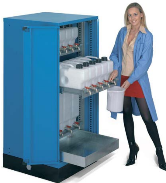
ORD. NO. F AE 8058 42 04 Cabinet dim. mm 717x750x1600 h. Complete with: 3 full extension retractable shelves (200 kg), 4 plastic cans 25 litres capacity, 10 plastic cans 10 litres capacity, 1 retractable safety tank for oil 40 litres capacity, 1 safety tank for oil 77 litres capacity, 2 plugs for tank. Total useful capacity of the cabinet: 200 litres Total capacity of safety tanks for oil: 117 litres
