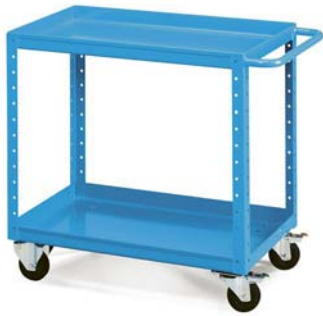
ORD. NO. Dim. mm F CR 0091 00 04 920x510x810 h Trolley with 2 standard rubber swivel wheels with brakes and 2 standard rubber fixed wheels Ø 100 mm. LOAD CAPACITY: 150 KG
