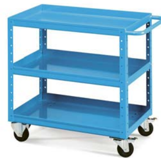
ORD. NO. Dim. mm F CR 0091 01 04 920x510x810 h Trolley with 2 standard rubber swivel wheels with brakes and 2 standard rubber fixed wheels Ø 100 mm. LOAD CAPACITY: 150 KG
